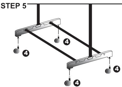
Finish up the assembly by inserting the castors part 4 into the bottom of the frame part 1. Pushing in with your hands only until they snap into place.
